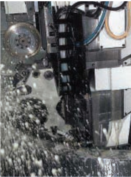
Special-design Gleason-Pfauter grinding head, used on Gleason-Pfauter profile grinders to speed production of internal ring gears.
